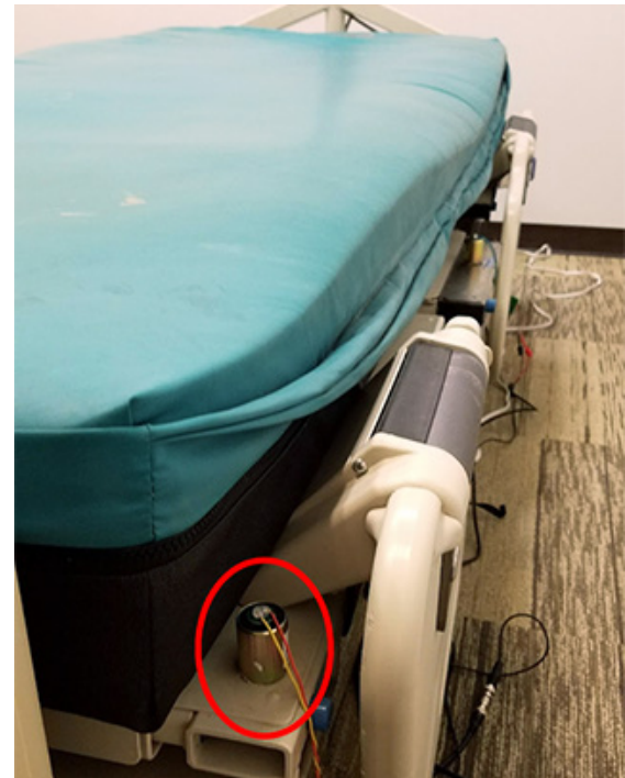
Source: Hae Young Noh The sensor attaches to the end or side of the bed.
