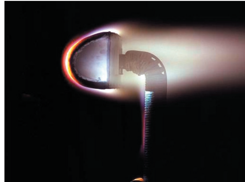
Lightweight ceramic ablator testing in Ames 60 MW Arc Jet Facility
