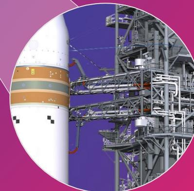
The more powerful **SLS exploration upper stage** requires a new umbilical on mobile launcher 2 along with enhanced propellant loading capabilities.
