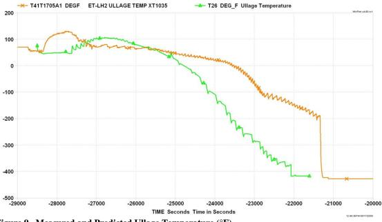
Figure 9. Measured and Predicted Ullage Temperature (°F)
