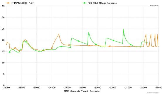
Figure 5. Measured and Predicted Ullage Pressure (psia)
