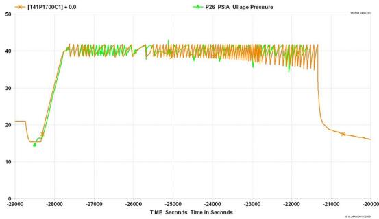
Figure 8. Measured and Predicted Ullage Pressure (psia)
