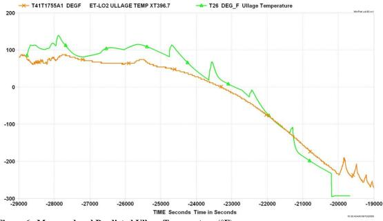
Figure 6. Measured and Predicted Ullage Temperature (°F)
