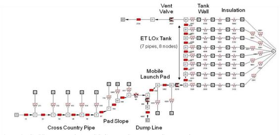
Figure 2. GFSSP Model of the KSC Ground System and Shuttle LOx Tank
