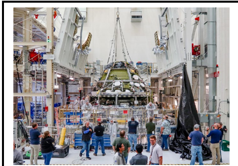
The second European Service Module was connected to the Crew Module to form the Orion spacecraft which will bring astronauts around the Moon and back during the Artemis II mission. The integration was done at KSC in Florida.
