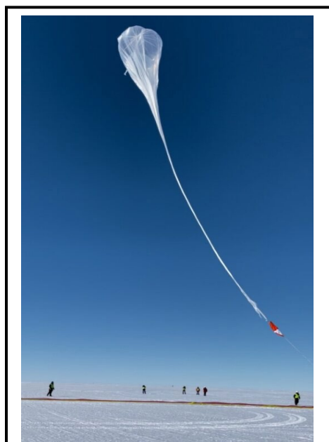
Long duration evaluation solar hand Launch (LAURA), shown here, hand-launched on December 11, 2023. LAURA is a NASA Balloon Program Office payload, intended to test instrumentation and power for a long-duration hand launch, to extend range and duration of hand launch missions.
