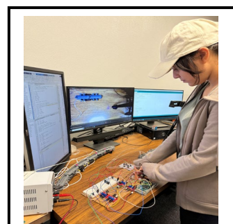
Ayla Valles, a graduate student at the University of New Mexico, is shown here working on the electro-pneumatic controller of the artificial muscle-driven snake robot for agile and energy-efficient limbless locomotion during planetary exploration.
