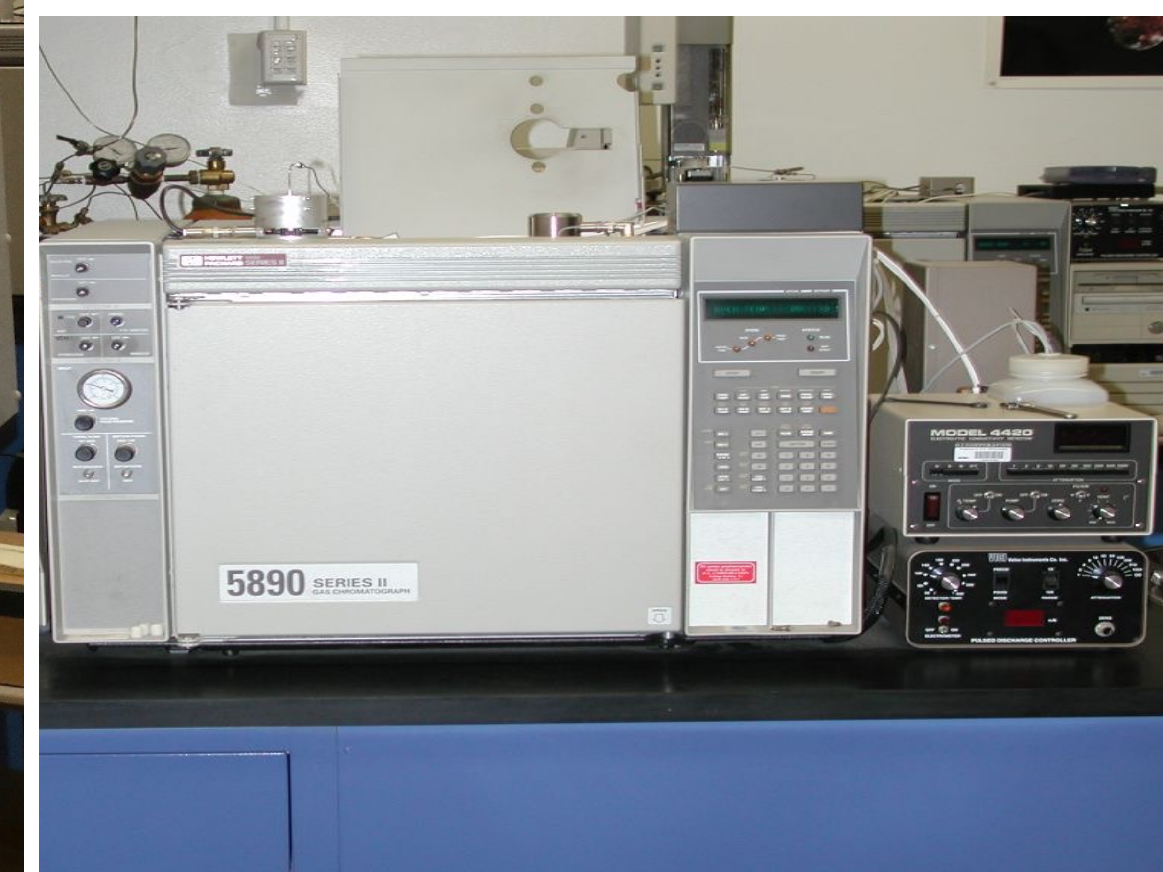
Detector (Hall) HP 5890 Gas Chromatograph Detectors: Flame Ionization Detector, Photo-Ionization, Pulse Discharged Helium Ion Detector (PDHID) and Electrolytic Conductivity
