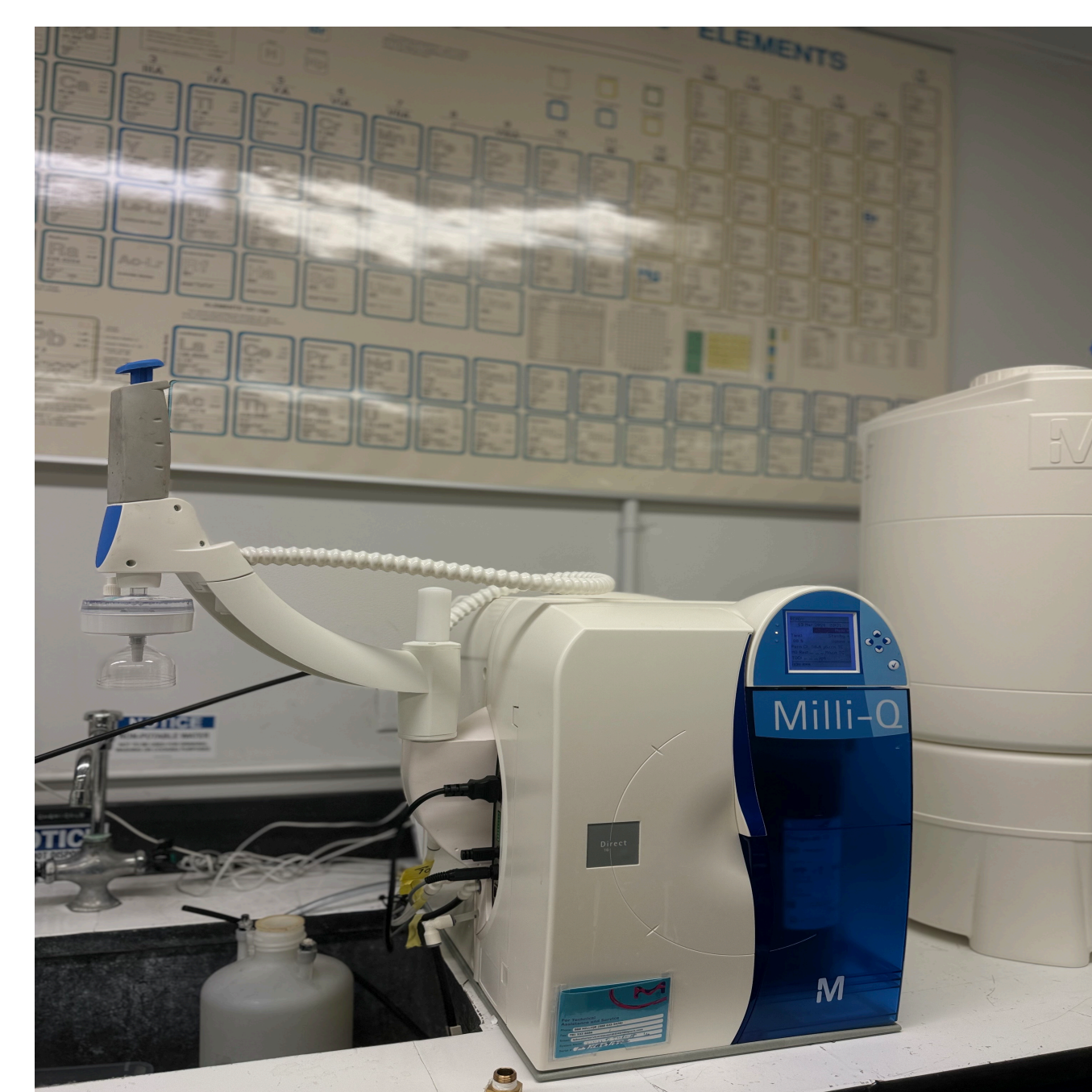
Milli-Q purified water system Good quality low TOC purified water
