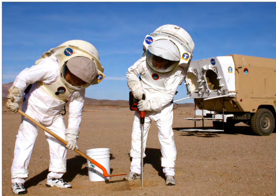
Figure 3. Field test of concept spacesuits and suitport interfaces in the Mojave Desert, California, at the U.S. Army's National Training Center at Fort Irwin. A modified Humvee, with aft suitports, was used as a pressurized rover simulator.
