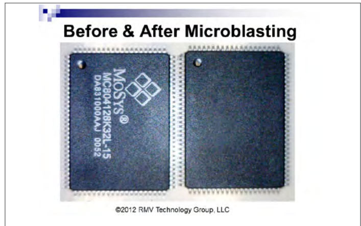
Figure 3. Suspect Counterfeit method of removing a component's lettering that does not show evidence of tampering.
