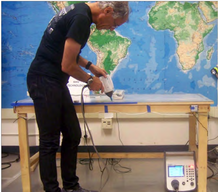
Figure 1. System Level Testing using IEC-61000-4-2
