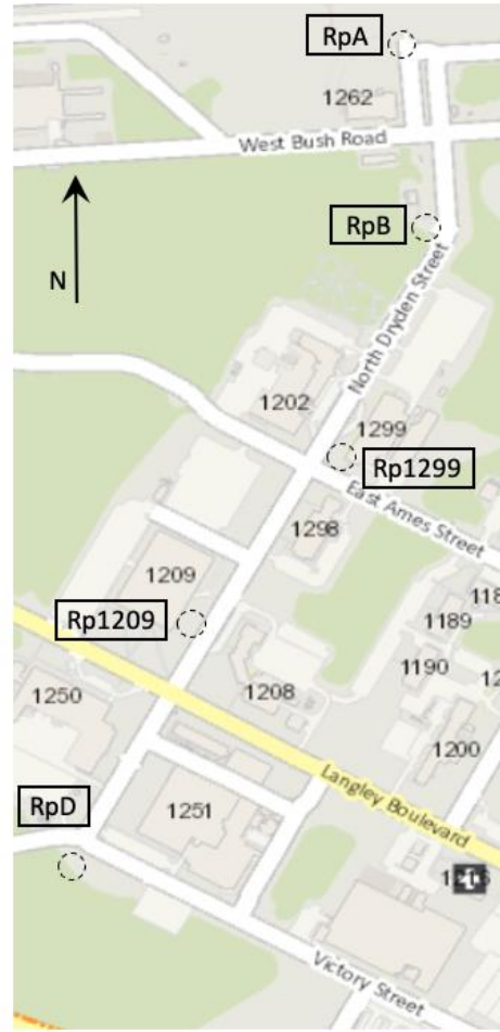
Figure 3. Flight range for operations over streets. Left: Satellite view showing polygonal keep-in geofence (dashed orange line) and waypoints (yellow circles) of the primary flight range. Yellow boxes contain the waypoint designators used in the flight plan. Right: Street view showing rally points (e.g., RpA, dashed circles) along the flight range. © Satellite map data: 2020 Google. Street map data: NASA
