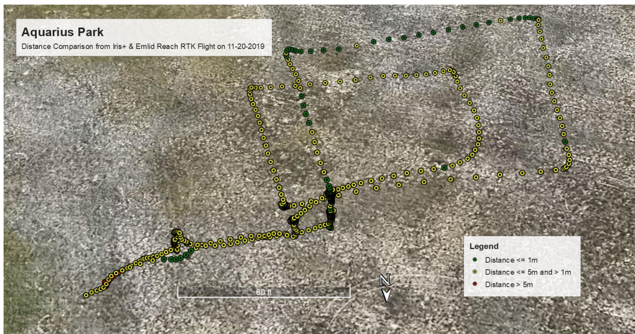
Figure 7 - Difference between RTK and basic GPS solution
