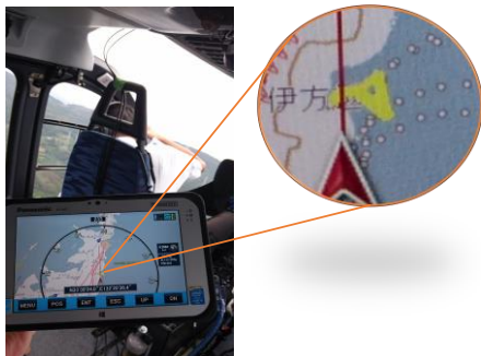
Fig. 11 Onboard D-NET portable system view. UAV area is shown in yellow, and the present helicopter position is shown by the red arrow.
