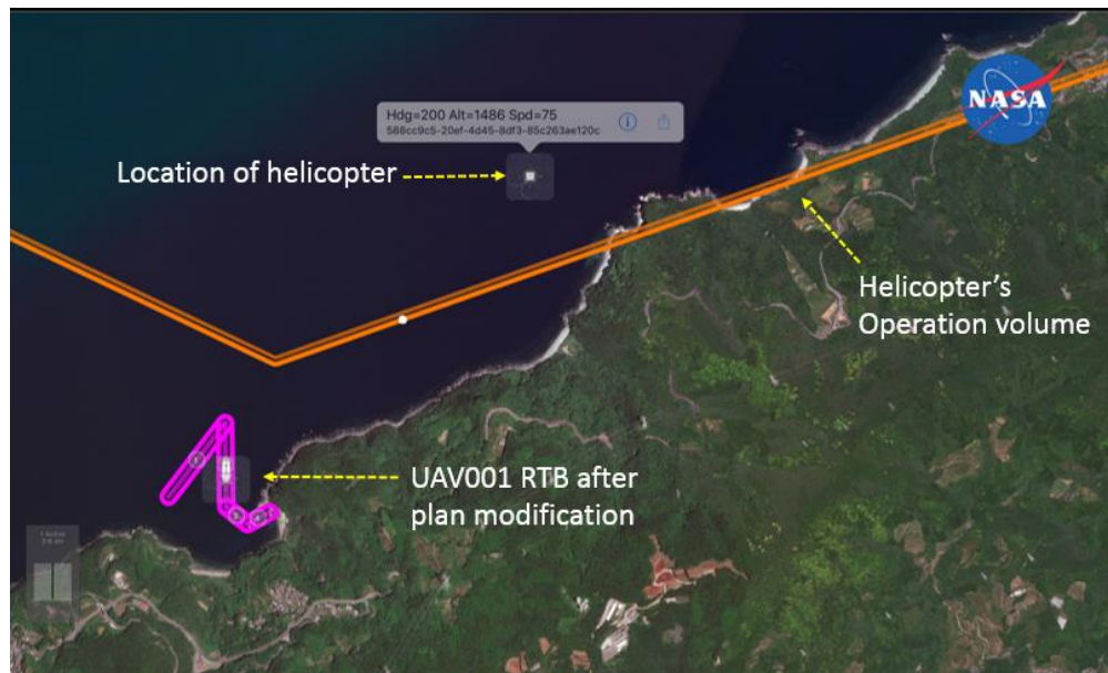
Fig. 15 Helicopter's operational volume, location and UAV001 modified flight plan
