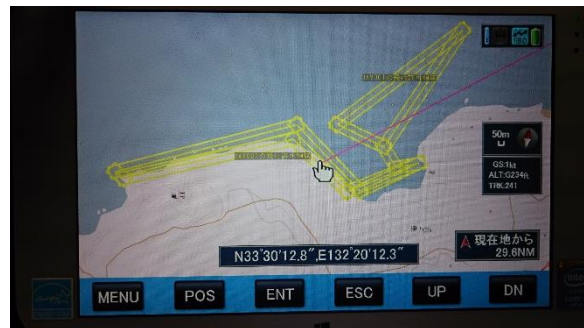
Fig. 12 Sample zoom-in of the UAV flight zones as seen onboard D-NET portable system. The yellow areas represent the airspace assigned to UAVs.
