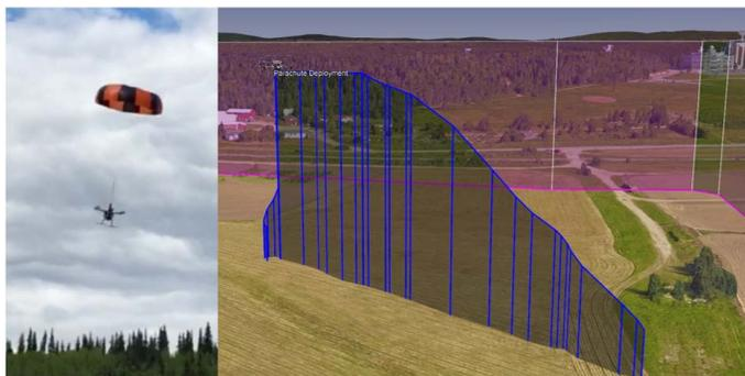
Fig. 4. Parachute deployment as part of contingency response (left) and associated flight profile and operation volume data (right)
