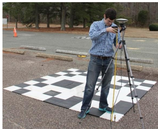
Figure 7: The RTK base station is mounted on a tripod and positioned over a surveyed location using a plum-bob.
