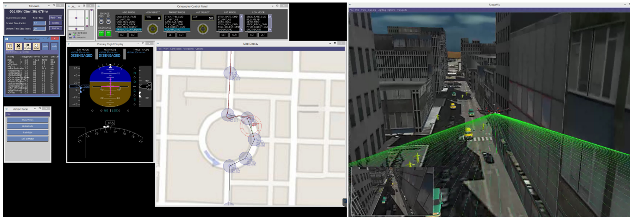
Figure 4. Ground station interface (left), path traveled by aircraft (center), aircraft navigating narrow urban street in Indianapolis, IN (right)
