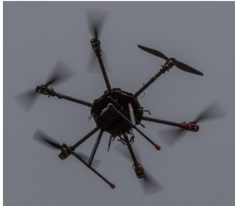
Figure 5. Tarot X6 in Hover with Right Center Motor Shut Down.
