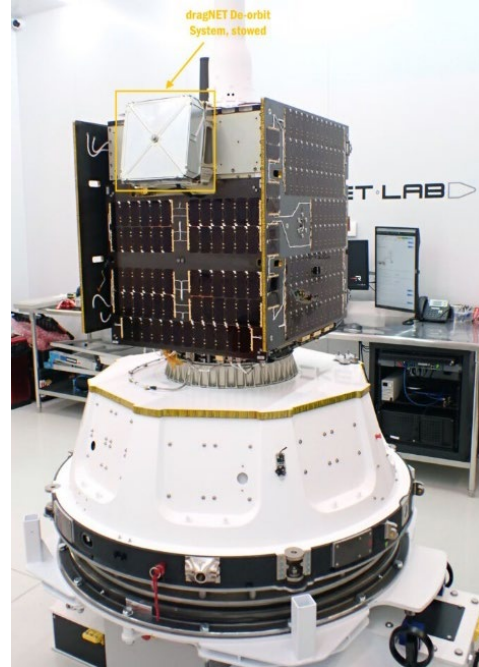
Figure 13.6: {top} The dragNET module. {bottom} dragNET module attached to the GAZelle satellite prior to its launch in late 2022. Credits: MMA design.
