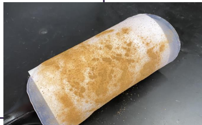
1-100 μm scale cinnamon adhered to gecko roller in ambient pressure proof of concept
