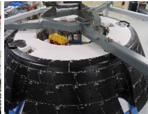
Forward Bay Cover Tile and FRSI Bonding Complete
