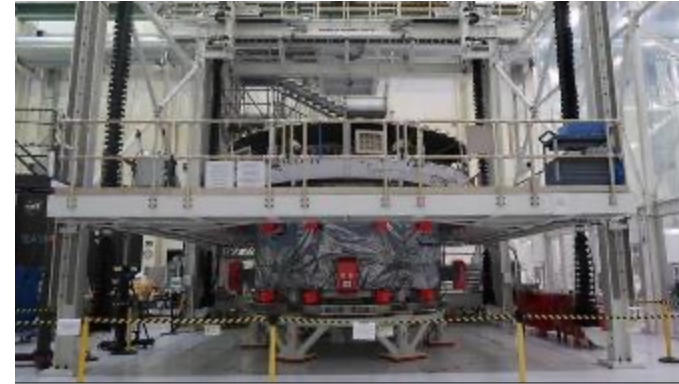
Crew Module Adapter and European Space Module Mate
