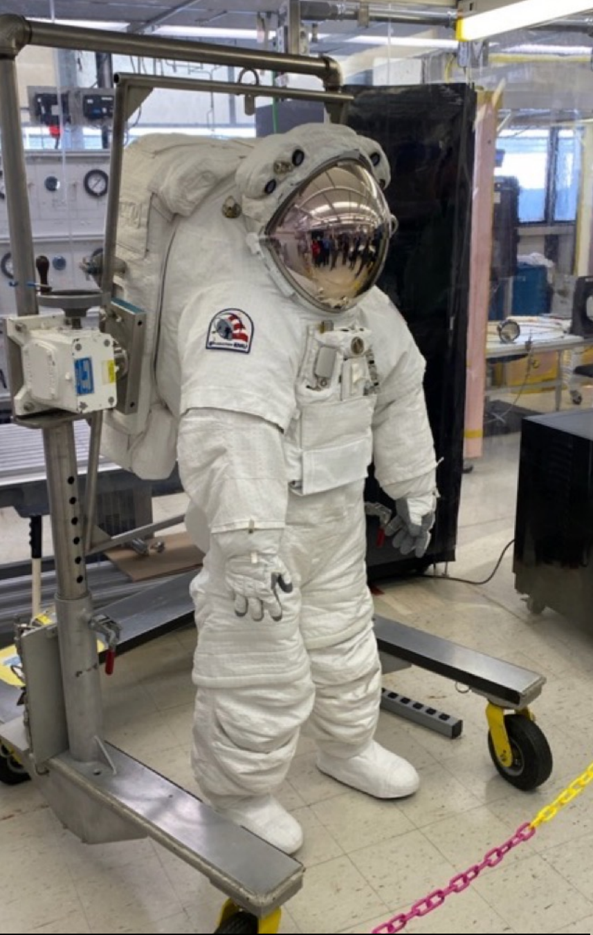
PRESSURE TESTING OF NASA'S FULLY ASSEMBLED EXPLORATION SPACESUIT
