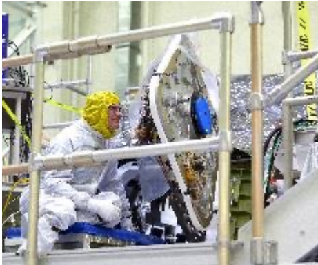
Artemis II Slide Hatch in Acceptance Testing
