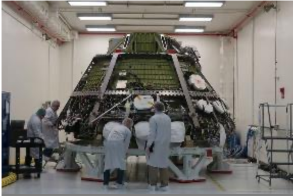
Crew Module ECLSS Bay Components Installed
