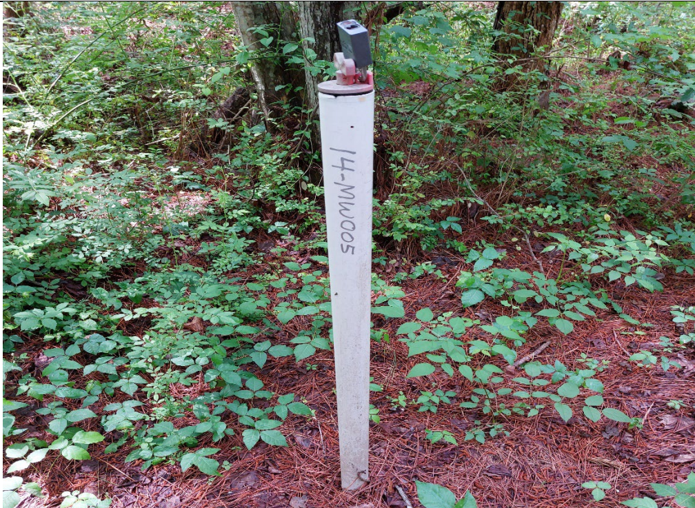
View of 14-MW005. There is no protective casing installed for this well due to the location.
