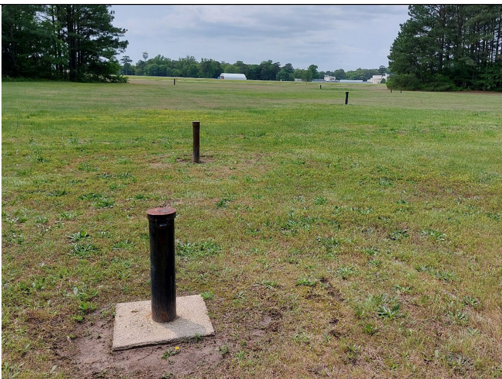
Date: 5/17/2023 View: Southwest Photographer: J. Martone (Tetra Tech; contractor for NASA) Standing adjacent to FFTA-MW102D looking across the site back towards the abandoned taxiway. Several other FFTA monitoring well are visible in the distance.
