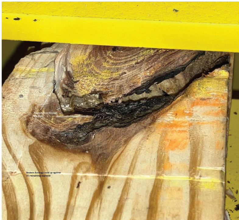
Figure 15: Fractured dunnage to show the extensive knot and fracture pattern along the knot.
