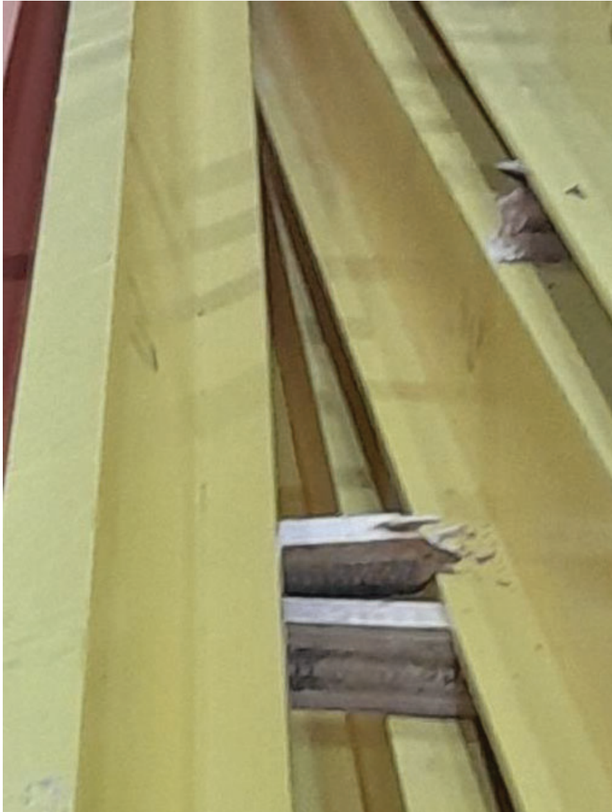
Figure 22: Broken dunnage and one of two beams that it supported.
