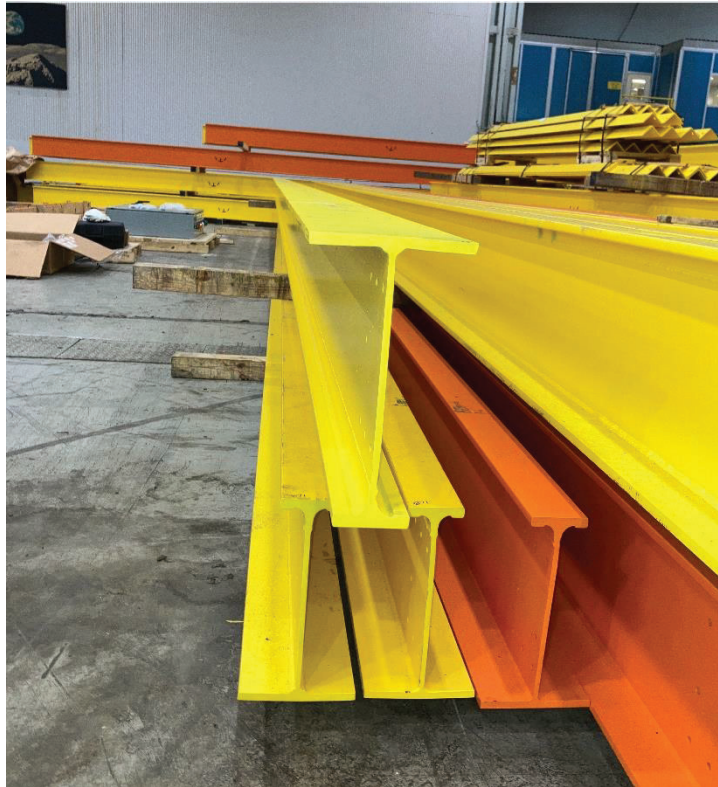
Figure 14: Beam upside down in stack.
