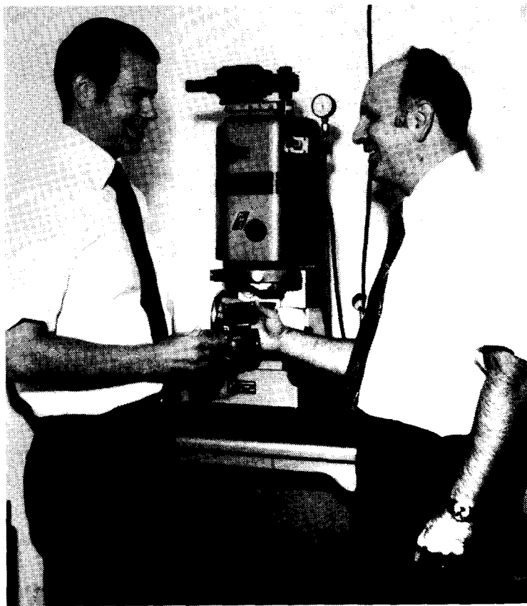
Faculty Fellow Dr. John J. Coy of the Rose-Hulman Institute of Technology (left), and Erwin V. Zaretsky, head of the Bearing and Gearing Section, measure surfaces of bearing elements using a surface tracer instrument called the rotary proficorder. (John Marton photo)
