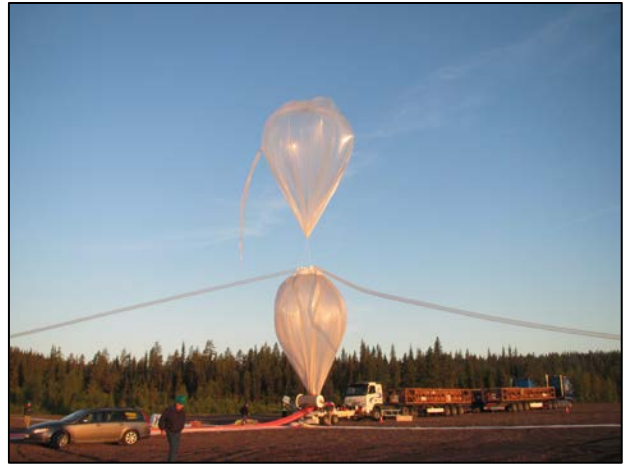
Figure 2-9: Tow Balloon atop Inflating SPB
