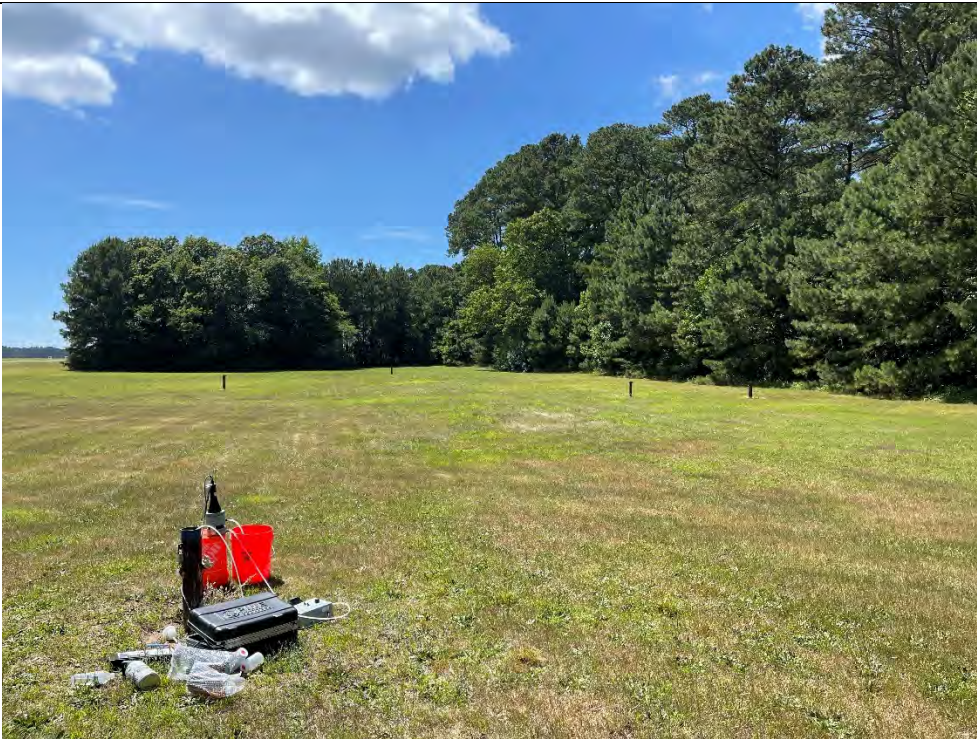
Groundwater sampling setup at FFTA.
