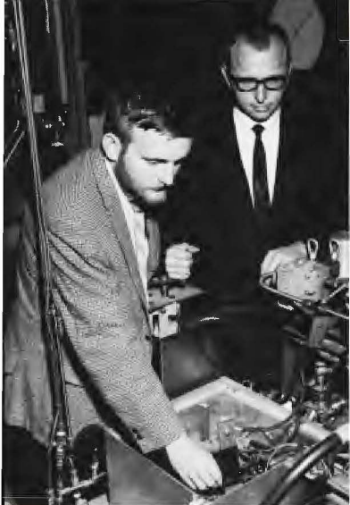
Robert Easter (left) and Paul Prokopius inspect a rig which tests fuel cell water rejection dynamics.
