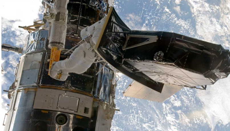
Astronaut Andrew Feustel delivers the Wide Field Camera 3 to the Hubble Space Telescope. Major process improvements were made to supply optical filters for the cameras and other NASA imagers. Source: NASA
