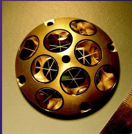
The Laser Retroreflector Array (LRA) is a passive optical instrument which helps provide measurements of distances between orbiting or landing spacecraft. Credit: NASA
