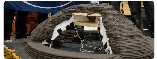
3D printed model of a lunar habitat created by Pennsylvania State University as part of NASA's 3D-Printed Habitat Challenge.
