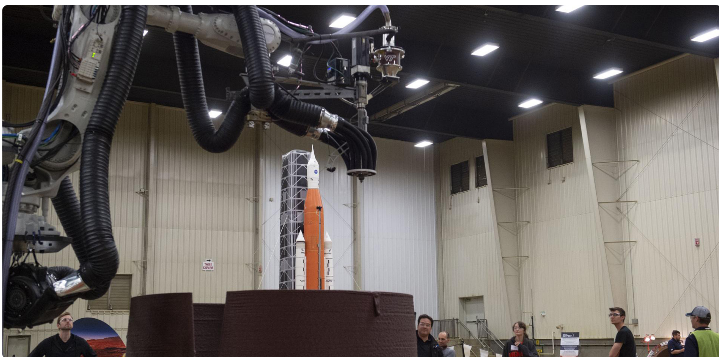
Team AI SpaceFactory's printer autonomously inserts a window into their 3D-printed subscale habitat structure at NASA's 3D-Printed Habitat Challenge, held at the Caterpillar Edwards Demonstration & Learning Center in Edwards, Illinois, May 1-4, 2019 Credits: NASA
