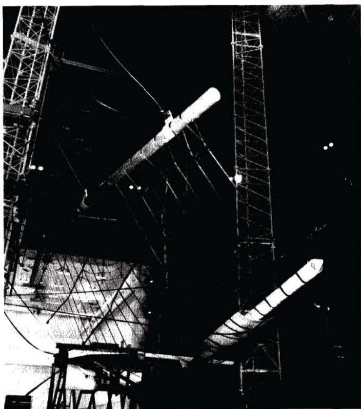
A mock-up Centaur shroud jettison test was successfully performed in the Space Power Facility at Plum Brook on October 4. The test was to demonstrate the acceptability of the catch-net system.
