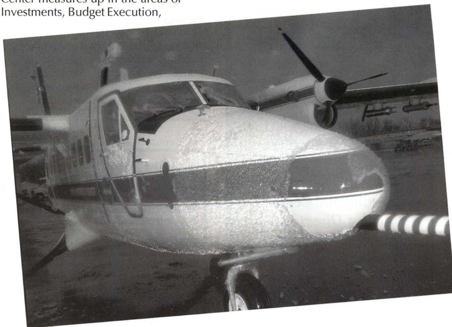
Reported during the Center Performance Review, the Supercooled Large Droplet Icing Flight Research program met its NASA Level 1 milestone. Data from the program is helping the FAA develop a better understanding of severe icing conditions, and enabling meteorologists to develop better icing weather forecasts.
