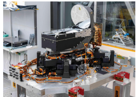
The DSOC flight laser transceiver shown here is stabilized by the vibration isolation platform (underneath the instrument), which was matured through the Flight Opportunities program. Credit: NASA/JPL-Caltech
