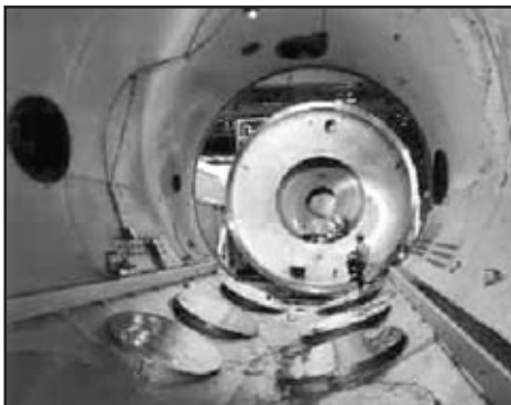
An inside view of Tank 5, which is 4.6 m in diameter by 19.2 m in length. The chamber has a pumping speed in excess of 3,500,000 liters per second.
