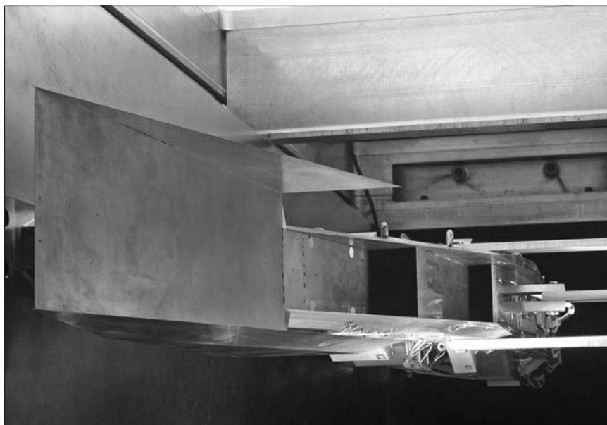
IMX model mounted in Glenn's 1×1 SWT.
