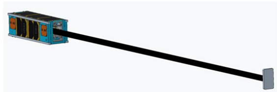
Figure 6.5: GPX-2 CAD image with gravity gradient boom deployed. Credit: NASA.
