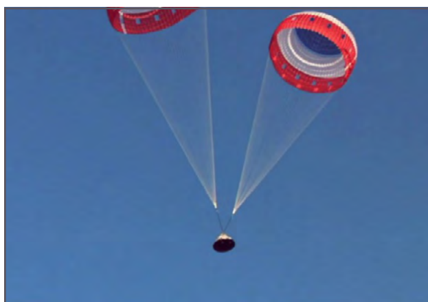
FIGURE 12. The Boeing Starliner descends under parachutes at the conclusion of the pad abort test
