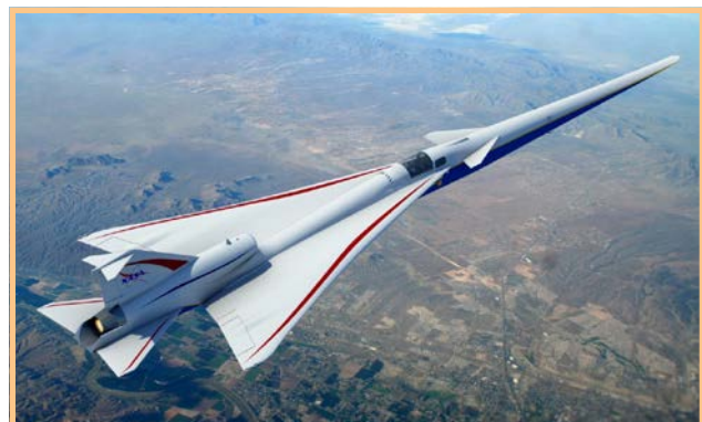
FIGURE 11. Artist conception of the X-59 QueSST Low Boom Supersonic Flight Demonstrator Aircraft
