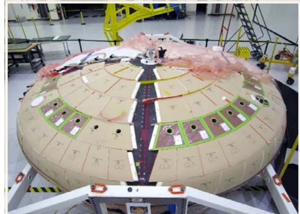
FIGURE 6. Avcoat Block Heat Shield Installation Underway
