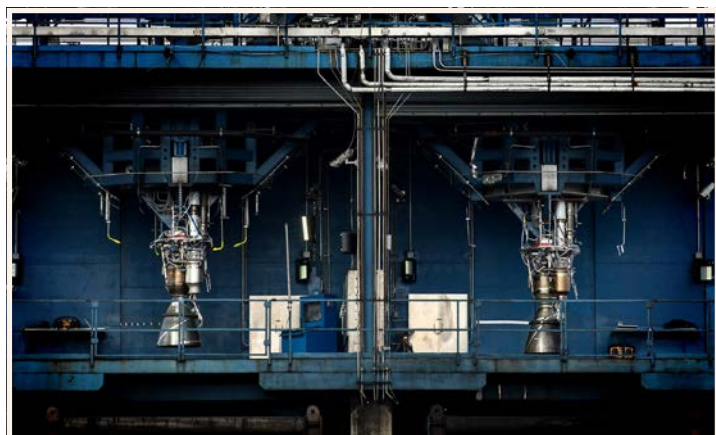
FIGURE 7. SpaceX's Merlin 1D Full Thrust Testing
