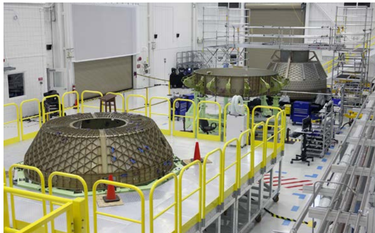
Figure 9. Boeing CST-100 Structural Test Article Being Assembled at KSC
