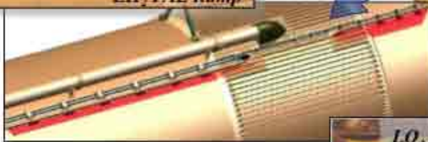
LO 2 and LH 2 PAL Ramp Elimination (Debris Mitigation)
