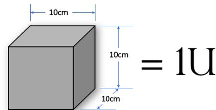
Figure 2.5 - CubeSat Dimensions.
