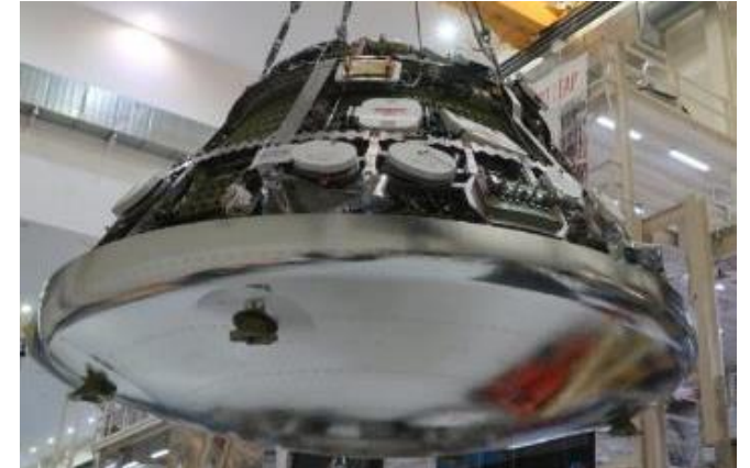
Integration of Crew and Service Modules for the Artemis II Orion Spacecraft
