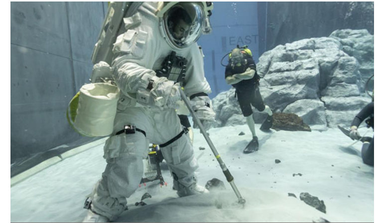
Spacesuit and hardware tests on the simulated lunar terrain on the Neutral Buoyancy Laboratory (NBL) pool floor
