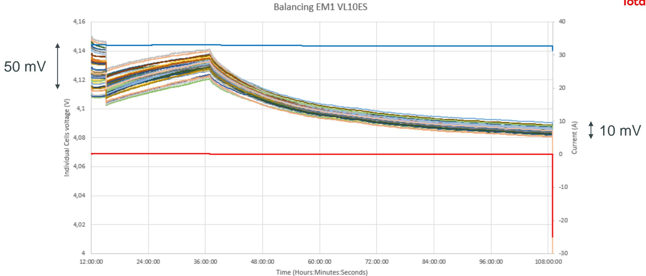
SBS capability : Cell to cell voltage spread criteria reaches in less than 48 hours
