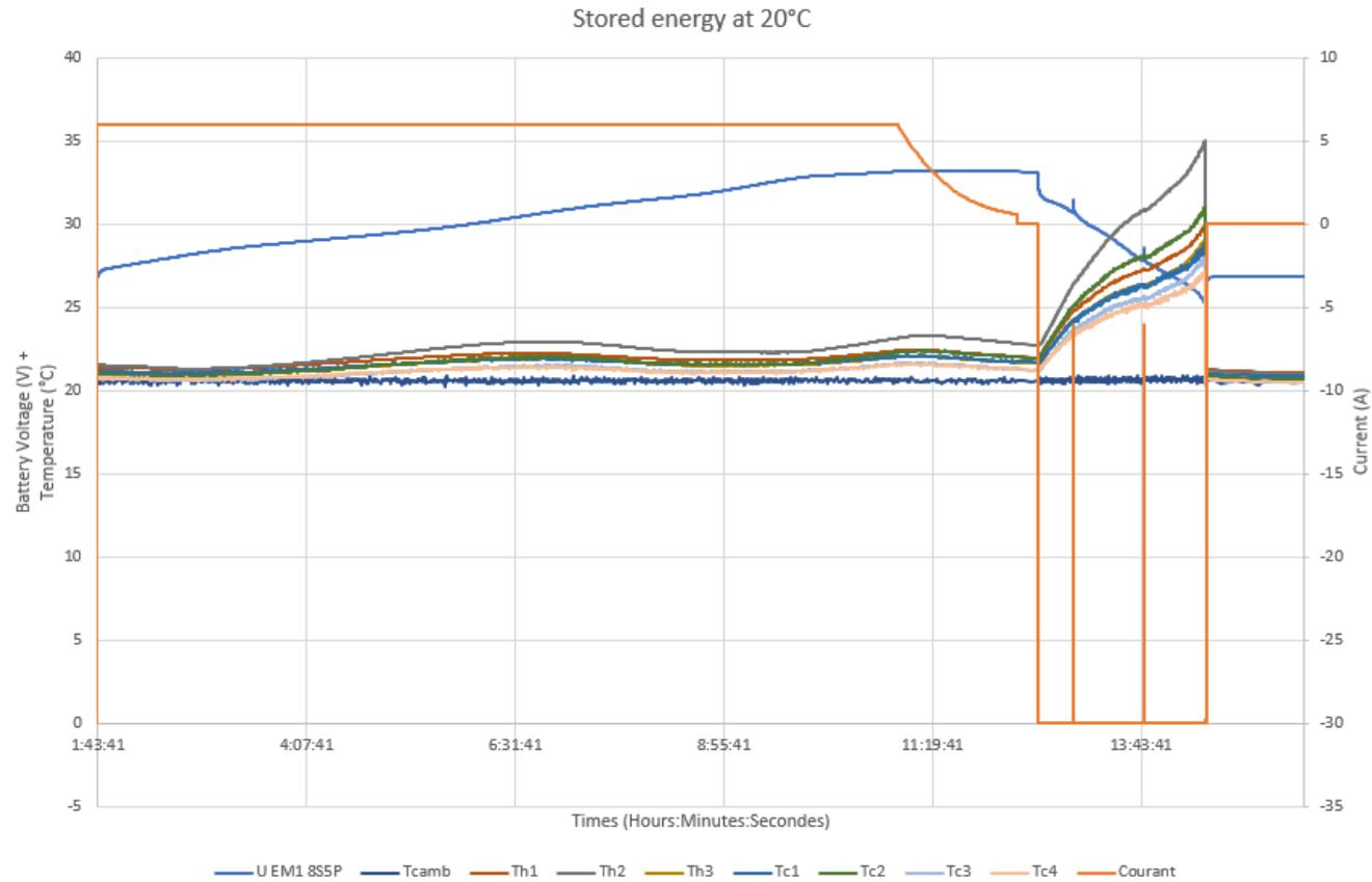
20°C capacity check with internal resistance checks.
