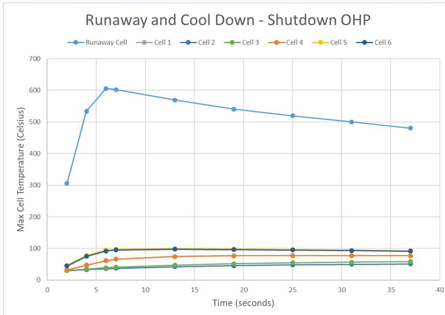
This scenario represents the worst case condition in which the OHP is *completely non-functioning* during the *entire* thermal runaway and cooldown event.
