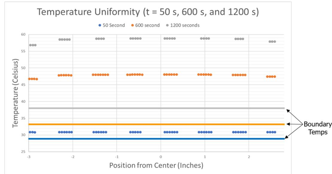
Results shown are for GA cells with a boundary temperature varying from 28 to 38 °C.
