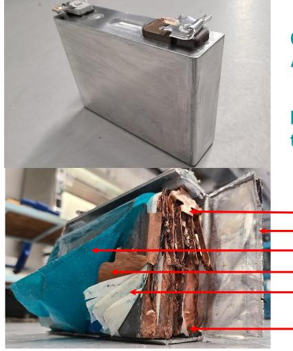
60Ah – NMC-based lithium ion cell (2014) Aluminum hard-cased prismatic cell
