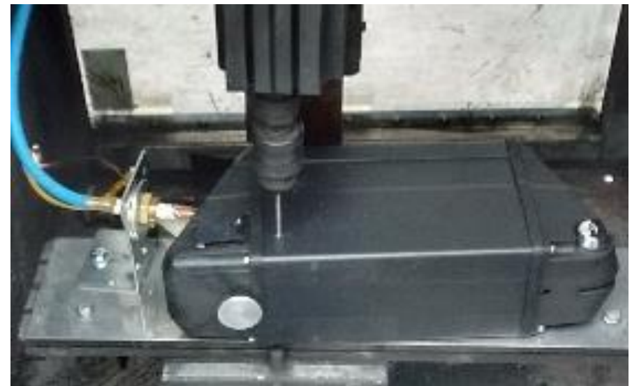
6 welds on trigger cell (normally 4)
