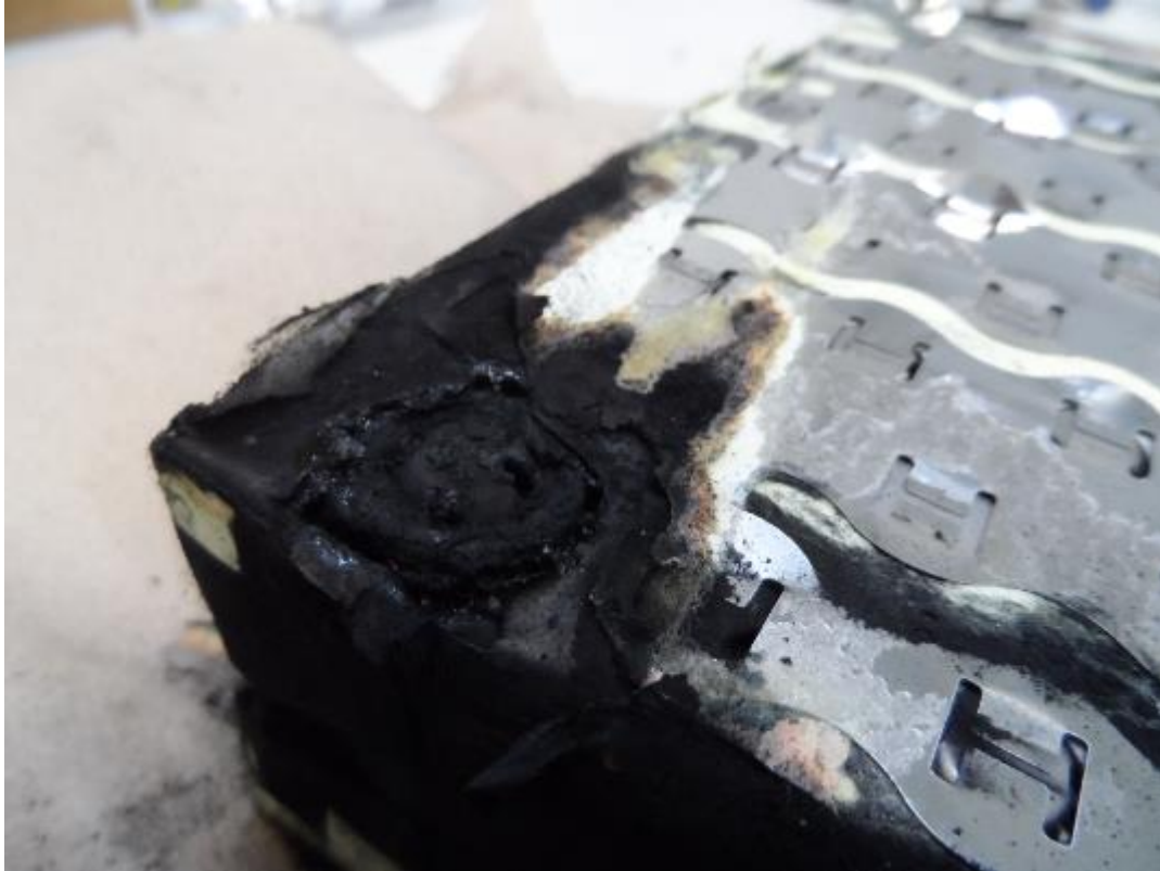
Nickel Cladding can separate from venting cell isolating electrical energy available for thermal runaway propagation
