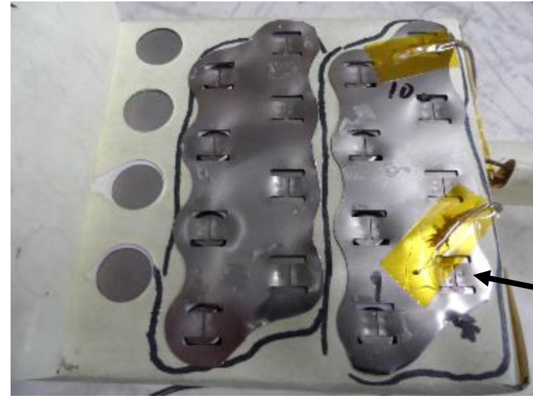
6 welds on trigger cell (normally 4)
