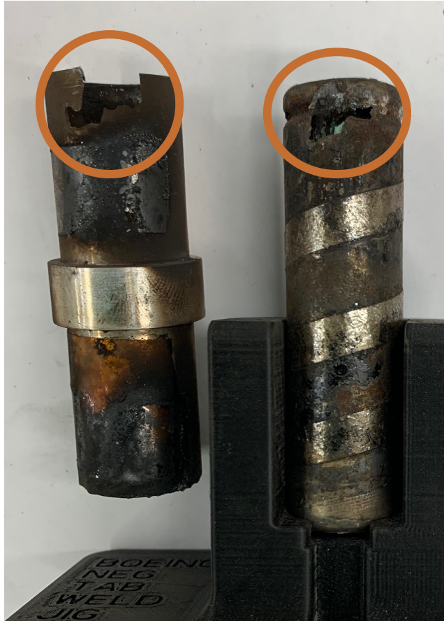
Spin groove & Sidewall Rupture with collar perforation
