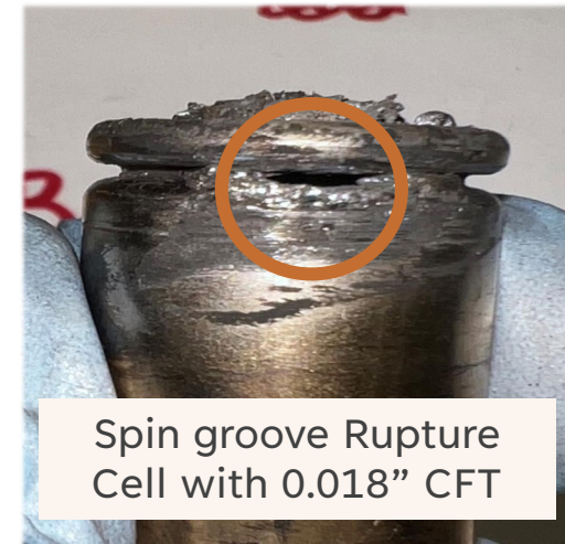
Spin groove and Sidewall Rupture Cell with 0.018" CFT
