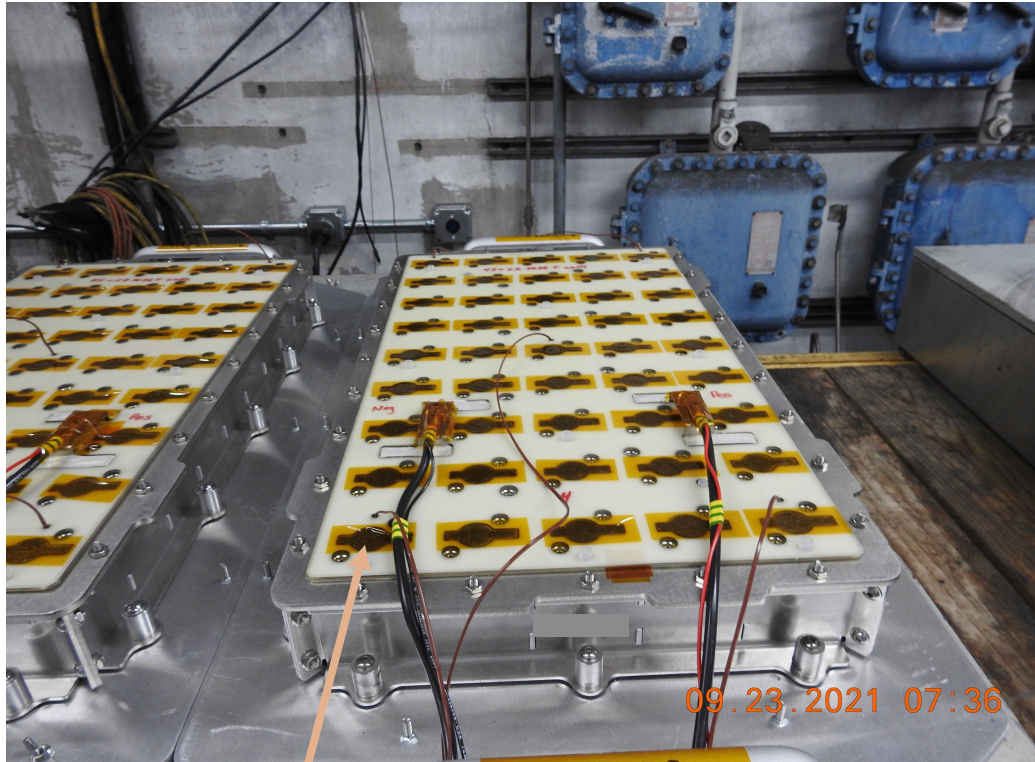
Mica covers to protect adjacent cells from ejecta
