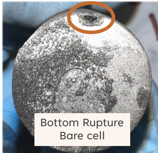
2x Bottom Rupture Cell with 0.012" CFT
