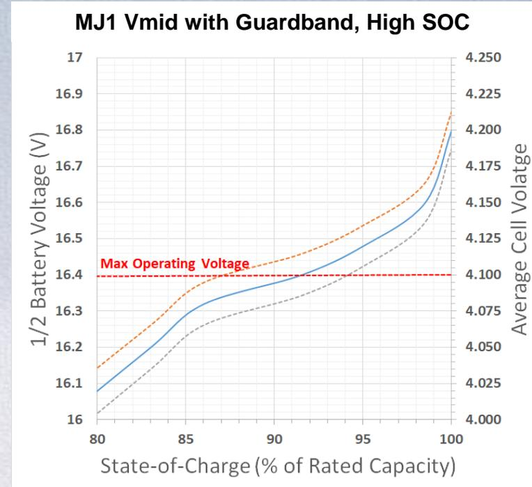
0.057 V Guardbands provide margin for ~ +3% and -5% SOC variance at high SOC
