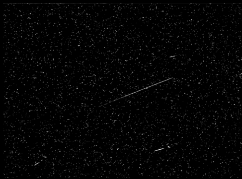
CMOS Imager under high proton flux irradiation
