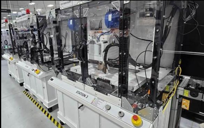
Pack Acceptance Testing (HASS-like stress test) performed over auto-dunk tanks
