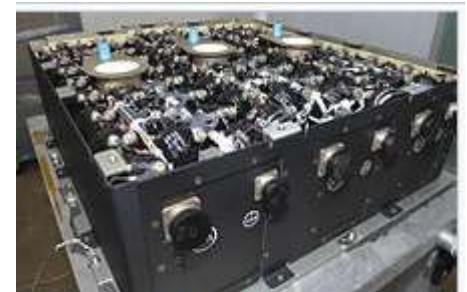
Nickel-Hydrogen batteries for Hubble [1]
