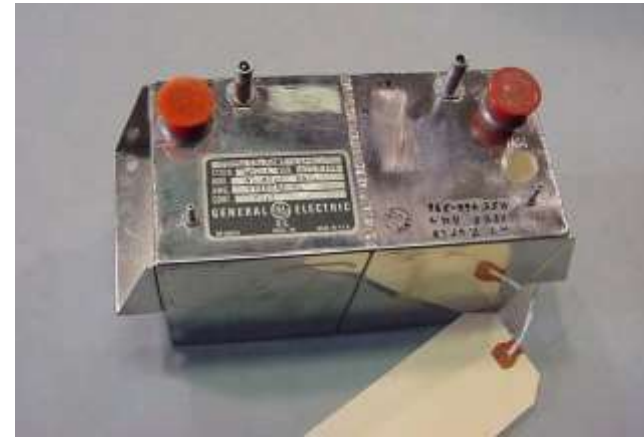
Silver-zinc battery, made by General Electric, was the only power source for the Corona satellite's film return capsule
