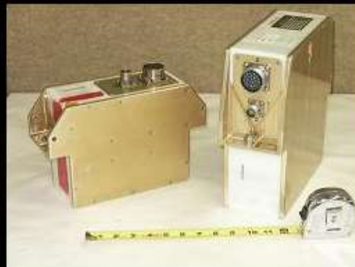
7 Ah and 10 Ah System Batteries with Heaters
