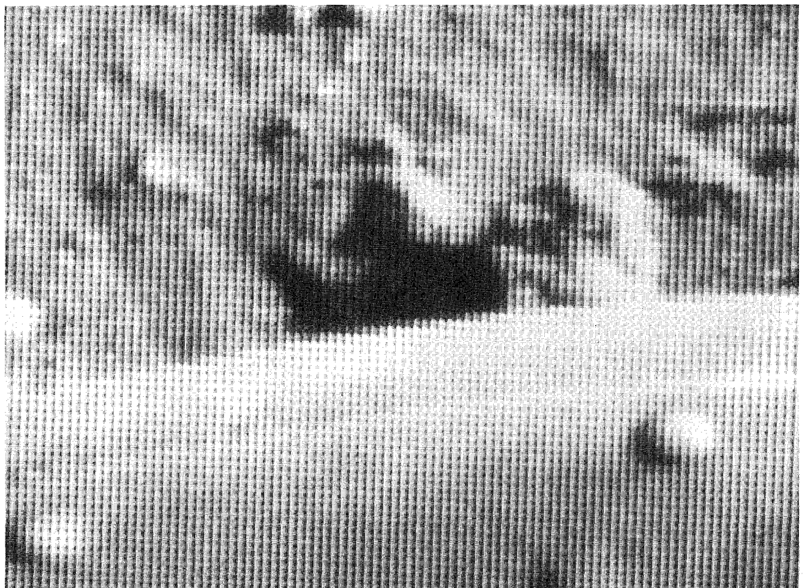
Figure 2. A part of the first picture taken on the surface of Mars, and a greatly magnified region within that picture. Note that the picture comprises a large array of discrete spots which range in brightness from white to black.
