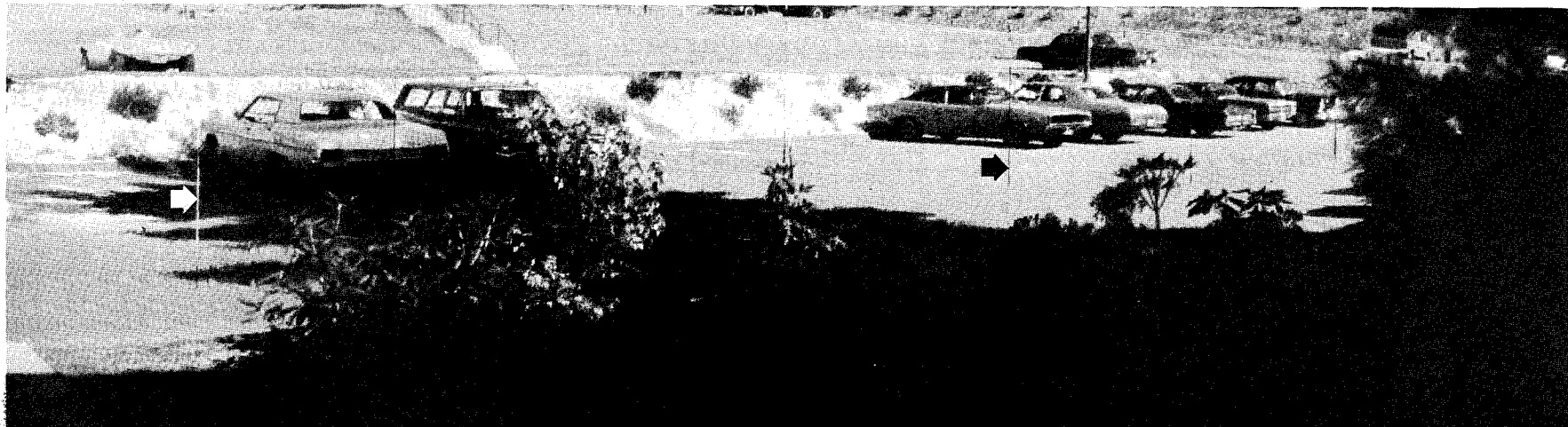
Figure 13. The first panorama taken with the Viking camera, a view of the ITEK parking lot in Lexington, Mass. The several vertical streaks, indicated by arrows, are not defects. They are the greatly distorted images of cars that drove by while the picture was being taken.
