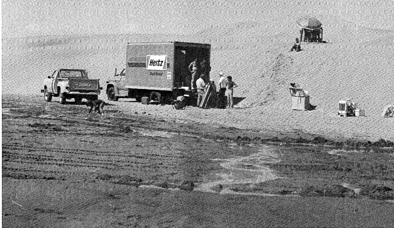
Figure 15. Operating the Viking camera at Great Sand Dunes National Monument, Colo. The camera is situated beneath the umbrella which protects it from the heat of the Sun. The supporting electronic equipment is in the rental truck.
