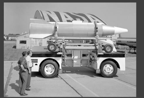
Image 32: A Lewis-designed hydrogen-oxygen demonstration missile (GRC–1959–C–51418).
