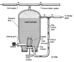
Image 199: Boiling Fluids Rig (NASA TM X-52320, Fig. 1).
