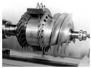
Image 113: A three-stage pump. The spiral-shaped inducer is to the right, the impeller to its left, and the single rotor stage is near the center of the photograph (GRC–1964– P–01638).
