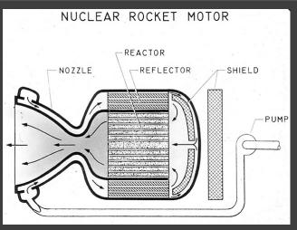
Image 24: Diagram of nuclear rocket engine (NACA CS-15514A).
