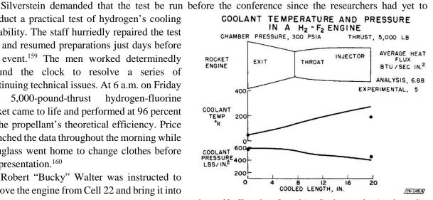
Image 33: Chart from Propulsion Conference showing the cooling characteristics of a regeneratively cooled hydrogen-fluorine engine (NASA TM X-67368, Fig. 22).
