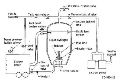
Image 135: Diagram of the Boiling Fluids Rig at C Site (NASA TN D–6361, Fig 3).
