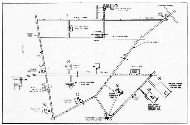
Image 2: Rocket Systems Area layout as it appeared in 1964. The dotted line denotes the route for a public driving tour of Plum Brook that October (NASA).
