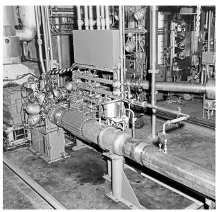
Image 188: Liquid-hydrogen test loop at A Site (GRC-1965-P-02010).
