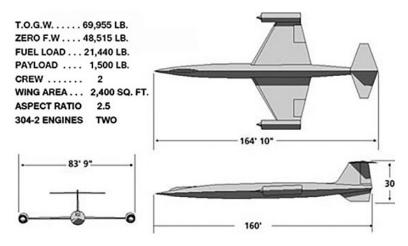
Image 28: Specifications for the CL-400 Project Suntan aircraft. The engines were located on the wings to compensate for the large hydrogen fuel tanks in the fuselage (NASA SP-4404, Fig. 34).
