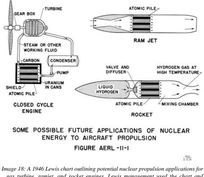
Image 18: A 1946 Lewis chart outlining potential nuclear propulsion applications for gas turbine, ramjet, and rocket engines. Lewis management used the chart and others like it to lobby for funding for in the coming fiscal years (GRC–1946–C– 15561).
