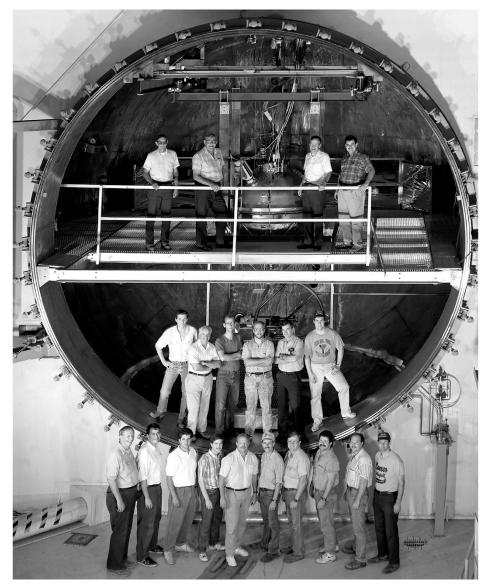
Image 178: Staff poses in the K Site vacuum chamber after the installation of a new slush hydrogen rig. A small propellant tank is installed between the four men on the upper level (GRC-1991-C-07453).
