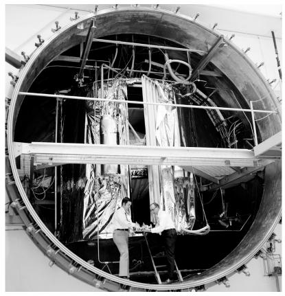
Image 156: Researchers with the CSTV, which is enveloped in a cryoshroud, in the Cryogenic Propellant Tank Facility (K Site) vacuum chamber (GRC-1974-C-03471).
