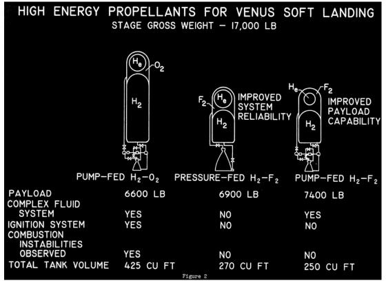
Image 94: Chart from 1962 demonstrating the superior performance of hydrogen-fluorine space vehicles. Fluorine increased payload weights and reduced the size of the tanks (NASA TM X–69544, Fig. 2).
