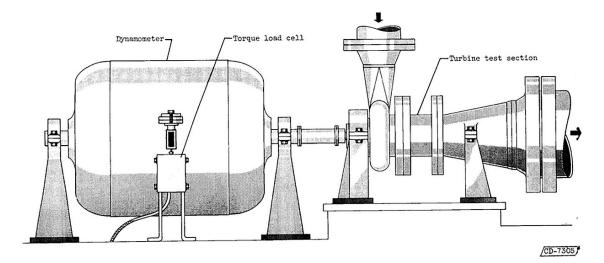
(a) Overall view. Figure 2. - Turbine test rig. Image 48: Diagram of the Pilot Plant's turbine test rig (NASA TM X-481, Fig. 2).
