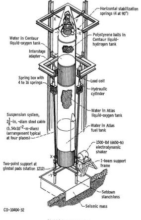
(b) Vehicle support system. Image 127: E Stand test setup configuration (NASA TM X– 1837, Fig. 2).
