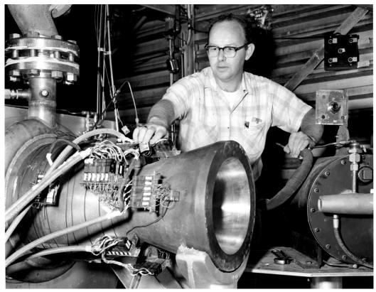
Image 73: James Coates inspects the 28,000-pound-thrust copper engine used for the nozzle heat transfer testing at J–1 in June 1962. The nozzle had a 5-inch-diameter throat that expanded to 11 inches and a coaxial injector to maintain stable operation and even mass flux and temperature (GRC–1962–P–01213).
