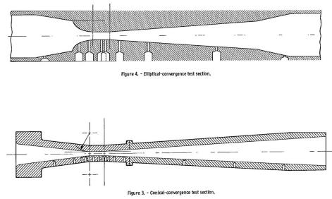
Image 159: F Site test sections used to study choked oxygen flow. The choking occurred in the restrictive throat section (NASA TN D–8169, Fig. 3-4).
