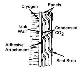
Image 146: Schematic view of SEMI insulation system (NASA Tech Brief 40–10646).
