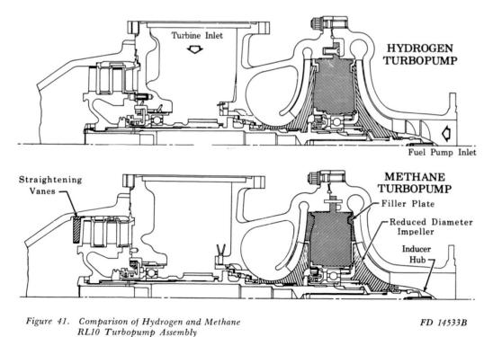
Image 133: Comparison of liquid-hydrogen and liquid-methane turbopump designs (NASA CR-72485, Fig. 41).
