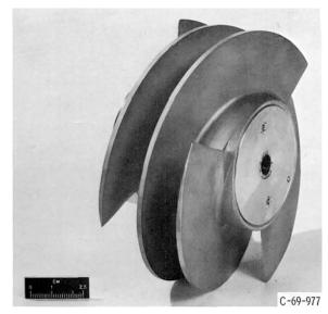
Image 134: An 80.6-degree inducer (GRC-1969-C-00977).
