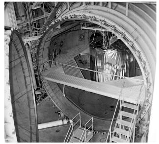
Image 234: Cryoshroud in the K Site test chamber (GRC–1971– P–01400).
