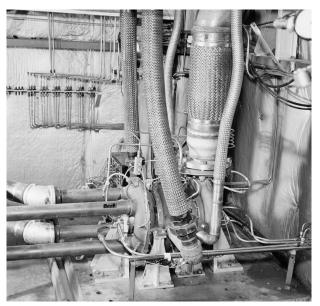
Image 215: Air brake at the Pilot Plant (GRC-2016-C-05134).
