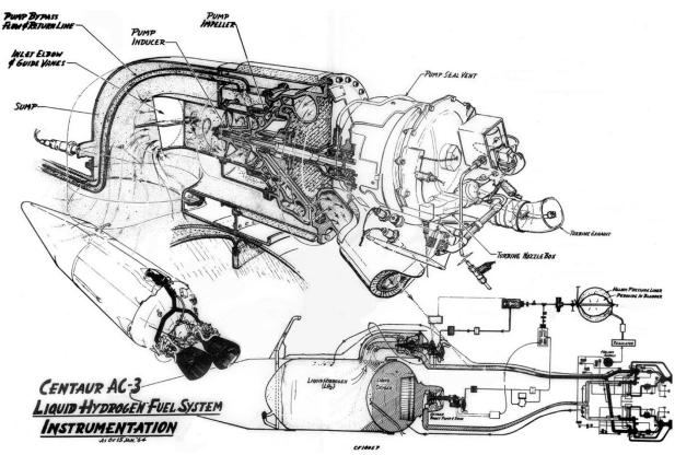
Image 142: Schematic drawing of the hydrogen boost pump for the Atlas/Centaur 3 (AC-3) vehicle (NASA).
