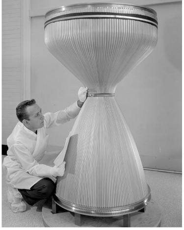
Image 105: A Lewis engineer examines the cooling passages on a converging-diverging nozzle for a nuclear engine. The nozzle had a unique 12 to 20 contraction ratio and 45-degree contraction half-angles<sup>450</sup> (GRC-1963-C-66545).
