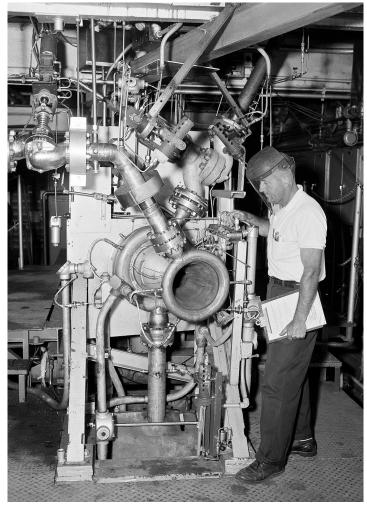
Image 141: A technician checks the installation of a steel engine in J–1 during November 1966. It was a 28,000-pound-thrust gaseous hydrogen-fluorine/oxygen (FLOX) engine (GRC–1967–P–01281).
