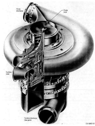
Image 109: Aerojet Mark III Turbopump. Several early missile systems used the Mark III, including the Navaho, Thor, Jupiter, Saturn I, and Saturn IB (NASA CD-10472-15).
