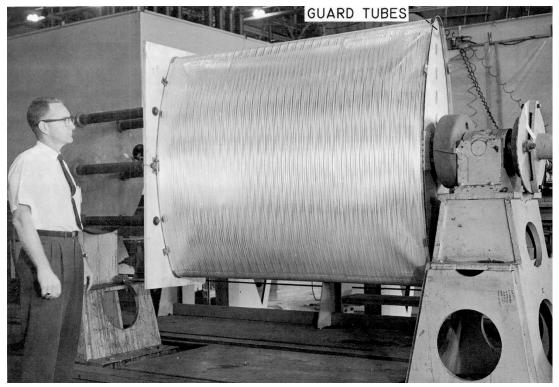
Image 77: A subscale insulated tank having a full-scale Centaur tank radius with a constrictive nylon wrap. NASA contracted Goodyear to fabricate four of the tanks and wrap three of them with a 160-strand-per-inch nylon constrictive wrap, and the fourth with a 64-strand-per-inch fiberglass binding<sup>339</sup> (NASA TM X–52004, Fig. 5).
