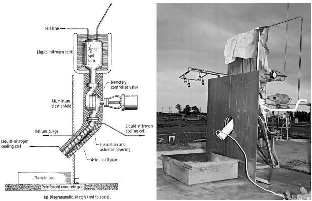
Image 119: Diagram of the spill test setup near J-5. The fluorine Image 120: Photo of the spill test setup near J-5. A vertical tank was at the top with a 4-inch pipe descending from the tank to approximately 2 feet above a 1-foot-deep and 3-foot-diameter pan that held the sample material. (NASA TM X-3118, Fig. 1).
